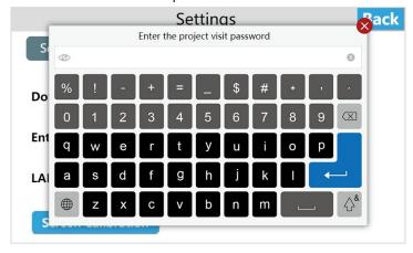
Click [Empty password], a pop-up "set up success", that is to clear the previous LAN password, users can access the HMI through the LAN (without entering any password).
